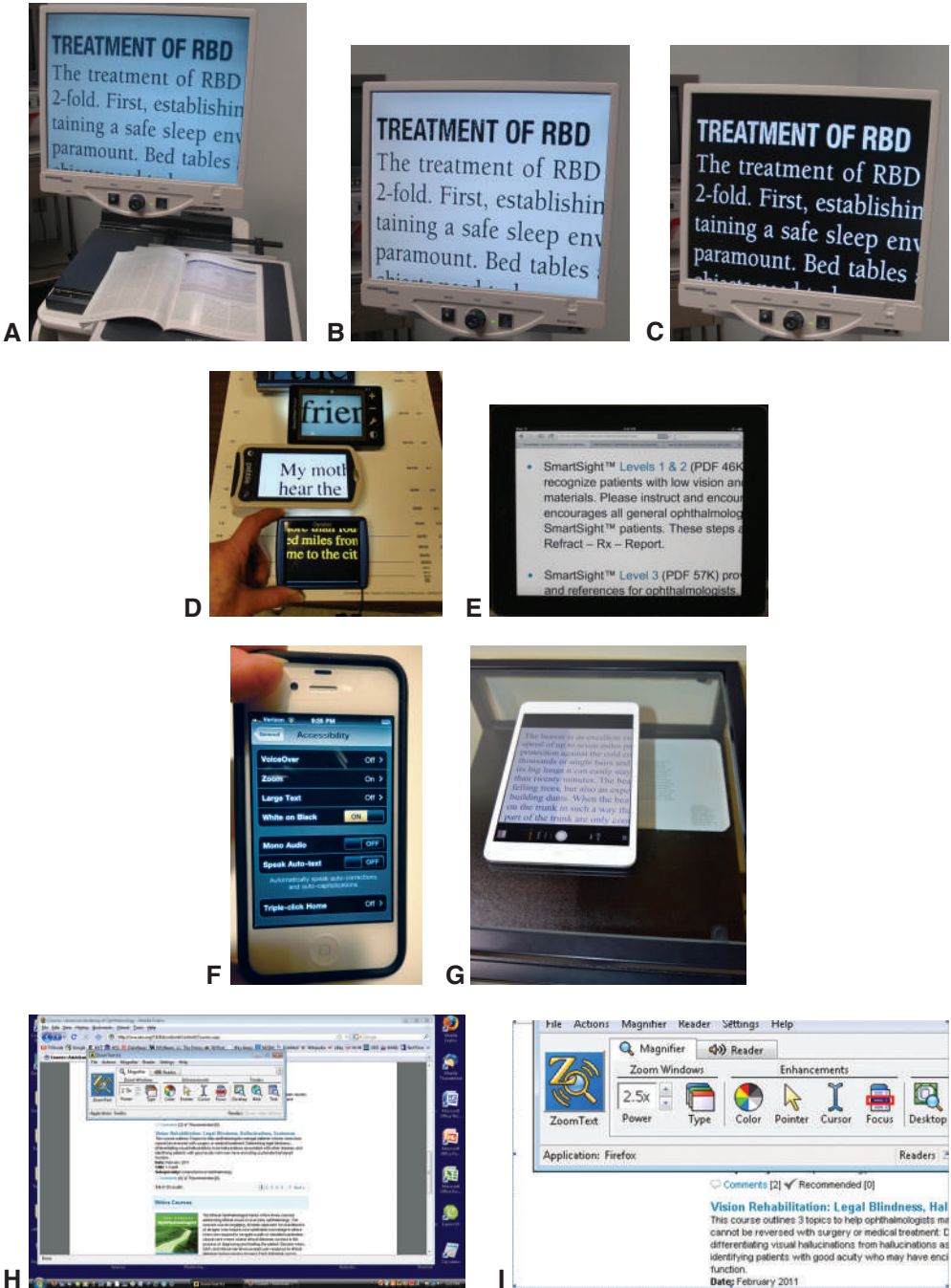
Figure 9-13 Electronic low vision aids. A , Desktop video magnifier. B , Same magnifier as in part A , in high-contrast mode. C , Same magnifier as in A , in reverse-contrast mode. D , Portable handheld video magnifiers. E , Tablet device used as a large-print e-reader. F , Smartphone accessibility features. G , Tablet device used as a video magnifier by placing on a glass desk. H , Standard-format Windows computer screen. I , Same computer screen as in part H , magnified using screen enlargement tools. (Courtesy of Scott E. Brodie, MD, PhD; Mary Lou Jackson MD.)
