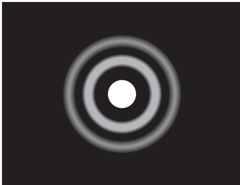
Figure 2-11 Diffraction pattern produced by a small circular aperture. The central bright spot is called an Airy disc. (From Campbell, C.J. Physiologic Optics . Hagerstown, MD: Harper & Row; 1974:20.)
