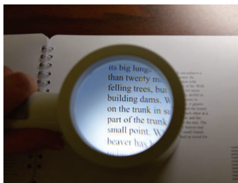
Figures 9-10 An illuminated stand magnifier placed flat against the page provides magnification, illumination, and stability. As with all magnifiers, the field of view decreases with increased magnification. (Courtesy of Mary Lou Jackson, MD.)
